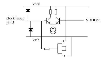
If the high clock level is greater than VDDD+0.5 V, a current will flow between the clock input & VDDD through the protection diode. This will affect the proper functioning of the ADC.
