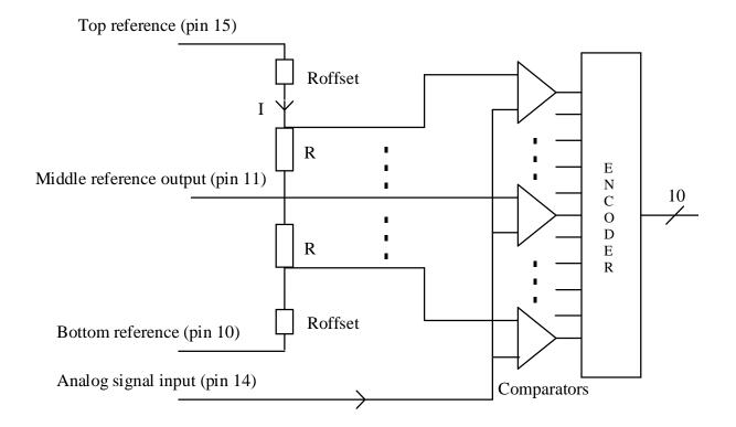
During the A to D conversion the analog input signal (pin14) is compared to voltage references by the means of voltage comparators (In fact these comparators are folding amplifiers).
