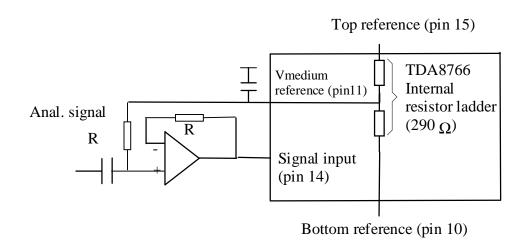
The R resistor in the op-amp loop compensates the offset due to the R resistor connected to Vmed. (R=1k $\Omega$ ; C=1 $\mu$ F)
