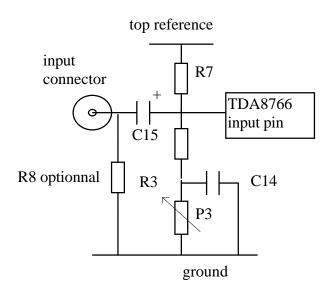
R3 is equal to the output load of the external signal generator. C14 allows ground connection between R3 and P3 in dynamic mode. Typical values when a 50  $\Omega$  signal generator is used are: R7=1K  $\Omega$ , R3=50  $\Omega$ , P3=5 k $\Omega$  (set at 2093  $\Omega$ ), C14=10 nF, then the current flowing through the resistor bridge is only 1.05 mA with a 3.3 V top reference. The solder print of an optional resistor R8 is provided in order to
