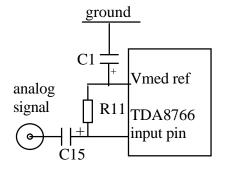
This method gives good results in the following domains : high common mode supply rejection (because both the voltage references and the input offset are derived from the same supply), very low noise level and low cost. R11\*C1 product must be high enough in order to avoid a coupling between the input signal and the medium reference. (C1=4.7 $\mu$ F for example) The offset on the input pin is: Vmed - (17 $\mu$ A\*R11)
