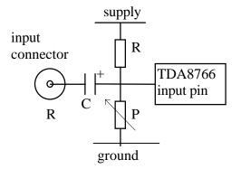
When a resistor bridge is used to provide an offset the current flowing through the resistors must be at least 10 times greater than the signal current (TDA8766 analog input current is 0 to 35  $\mu$ A) in order to guarantee the stability of the input offset. Consequently the resistive value of this resistor string must be below 8.5 k $\Omega$  (with a 3 V supply).
