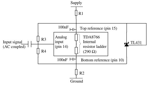
The (top - bottom) difference is set at 2.5V by the TL431, so the full scale input is set at 0.871\*2.5=2.18V. In addition the input offset is set at (Vtop+Vbottom)/2 by two equal resistors (R3 and R4).
