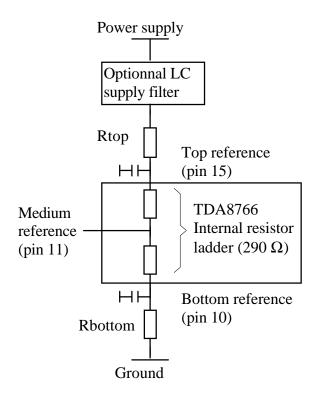
It is possible that the top reference equal the power supply voltage. So the Rtop resistor can be removed. An optional filter can be added on the analog supply (depending on supply noise level).
