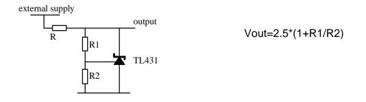
The power consumption of each TL431 is volontarily set higher than necessary in order to allow different ADC voltage supplies. See section 10: how to change the ADC supplies.
