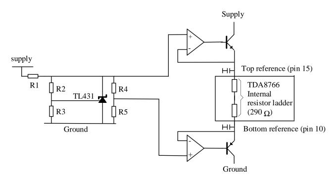
Operational amplifier with a low input offset should be used. The transistor types depend on the number of TDA8766G mounted in parallel. (7.5 mA typ. for one TDA8766G)
